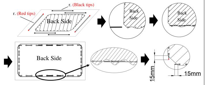
**Step 8:** Carefully and gently place the assembled frame on top of the screen material in the marked areas as shown below. Make sure to not allow the angle edge of the frame to come in direct contact with the screen material to avoid
