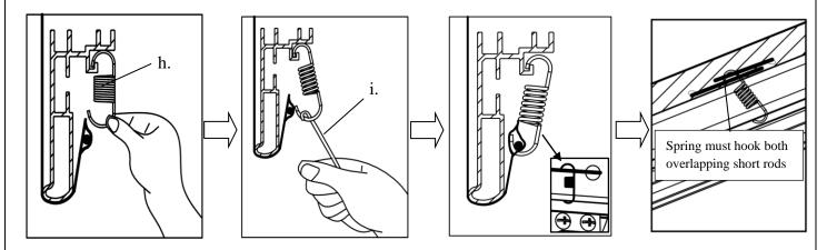
Begin by first attaching the center points on both vertical (left/right) sides, *steps 1-2*. Then the center points on both horizontal (top/bottom) sides, *steps 3-4*. Once all center points have been secured, make sure the screen material is still within the marked areas before proceeding to attach the next springs.
