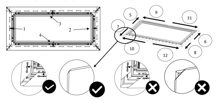
To avoid ripples forming in the material it is imperative that all of the corners are properly wrapped around the edges as illustrated in the check mark diagrams.
