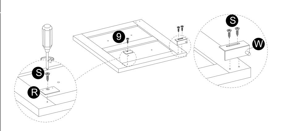
Attach hinge-top (W) to panel (9) with screws (S) correctly.
