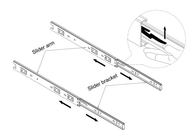
$\cdot$  Separate the slider bracket from the slider arm as per diagram.
