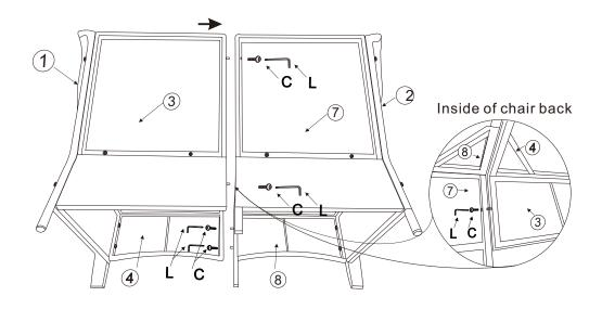
Step 5: Connect and secure both half chair together with 4 screws (C) by using allen wrench (L), two at the chair back and two at the front seat panel.
