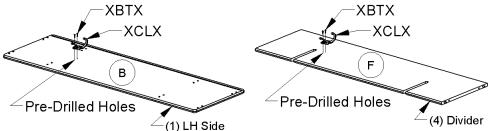
2. Assemble locker face down. Install <u>Shelves-E to LH Side-B</u> by aligning dowels in Shelves with dowel holes in Side. Ensure back groove is up on LH Side, and Shelf 'rounded edges' are down. Secure with 4-**XAUR** Decorative Screws with 4mm Hex Wrench provided.
