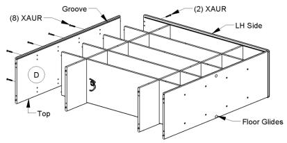
5. Install RH Side-C to Top, Bottom and Shelves by aligning dowels into dowel holes in RH Side. Secure with 8-XAUR Decorative Screws with 4mm Hex Wrench provided.
