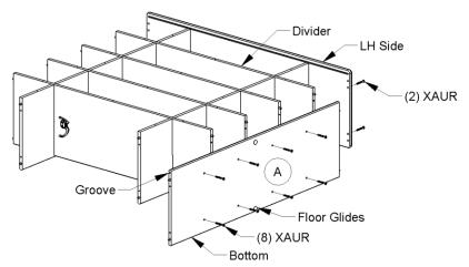
4. Align dowels of <u>Top</u>-**D** with dowel holes in LH side and 'partially' install with 2-**XAUR** Decorative Screws. Align dowels with each Divider to Top dowel holes and install 8-**XAUR** Decorative Screws. Tighten XAUR Screws to the LH Side.
