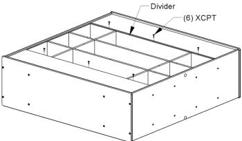
8. Install remaining 3-Backs in the same manner. Once all backs and screws are installed tighten all screws.
