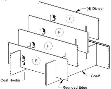
**DHCJX – Rev. B – 23 October 2019** 800-543-4149 507-342-5169 www.jonti-craft.com JonTi-Craft, Inc. 171 Hwy 68 P.O. Box 30 Wabasso, MN 56293 3. Align dowels of <u>Bottom</u>-**A** with dowel holes in LH side and 'partially' install with 2-**XAUR** Decorative Screws. Align dowels with each Divider to Bottom dowel holes and install 8-**XAUR** Decorative Screws. Tighten XAUR Screws to the LH Side.
