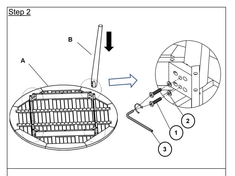
Attach Leg(B) to the Table Top(A) using Bolts( $\widehat{1}$ ), and Washers( $\widehat{2}$ ) with Allen Key( $\widehat{3}$ ). **Do not fully tighten the Bolts**.
