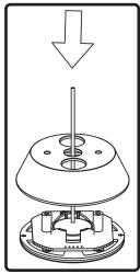
3. Place a pen or screwdriver in the bottom opening to dislodge the top touch panel.
