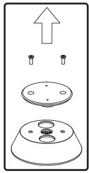
2. Remove (2) screws from the bottom of the remote control.
