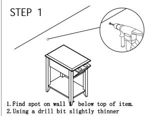
than anchor, drill hole into drywall.
