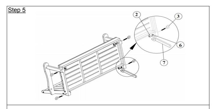
Connect Seat Panel (B) to Left Arm Panel (C) and Right Arm Panel (D) using Lock Nut (2) and Eye Bolt (3), Flat Washer (6) with Wrench (7) as shown above. **Do not fully tighten the Bolts.**
