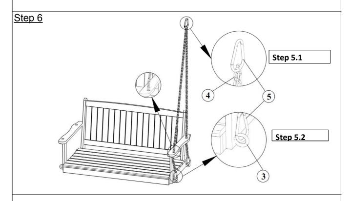
With assistance from your adult partner, turn right side up the assemble on step 4 as shown above **Step 5.1** Unscrew the connection on Carabiner (5) and loop the Chain (4) onto the Carabiner (5), then screw the connection shut as shown above
