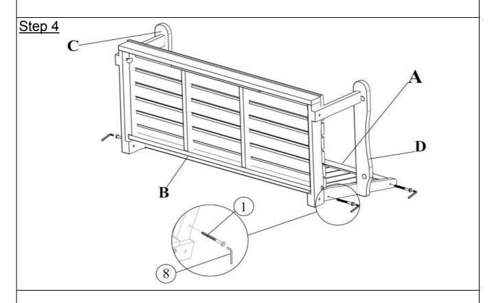
With the help of your adult partner, insert the tenon of the Backrest Panel (A) into the mortise of Left Arm Panel (C) and Right Arm Panel (D) of assemble in step 2.
