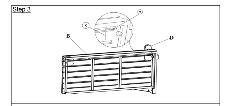
Secure the Seat Panel (B) to the Right Arm Panel (D) using Screw (9) and Allen Key (8) **Do not fully tighten the Screws.**
