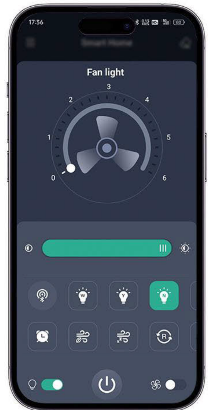
Step6 Turn on the pairing button. To ensure the app successfully connects with the device, click the "📶" button within 5 seconds after powering on the device. If the device flashes or beeps, it indicates that the phone and device have been successfully paired, and you can control the lamp through the app.
