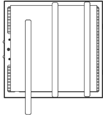
Place charcoal filter on back-side of baffle filter. And place filter brackets over charcoal filter and secure in place by tucking each end of bracket under the baffle filter frame. Re-install baffle filter.
