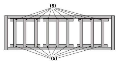
2. Next, attach the mattress base to the frame that you have already constructed. Attach the mattress slats to the inside faces of the bed ends using the fixing bolts [5]
