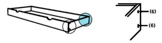
Install the drawer bottom support under the drawer by inserting the dowels [4] into its side openings, screw the pins [9] into the hole in the middle of the back and the front of the drawer, and the holes at the bottom of the bottom support - connectors [10], which we will tighten at the end after assembling the whole drawers.
