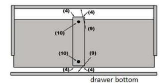
Finally, there is the drawer front, in which the pins [9] should be inserted from the inside. In the sides of the drawer, the connectors [10] should be placed, which must be tightened after joining the front with the sides. Screw the wheels to the edge of the drawer sides with screws [7] and the handles to the front.
