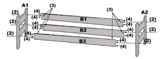
I. Start by constructing the slatted sides of your Atlas Convertible Toddler Bed and attach them to the starry front pieces of the bed. Place the wood dowels [4] in the side bars of the bed [BI, B2, B3], but leave the middle hole empty. Place the barrel nuts [3] in the opening on the side of the bars. Connect either side with the front panels of the bed [AI and A2] using fixing bolts [2] through the front sides into the middle hole that you left empty on the previous step.
