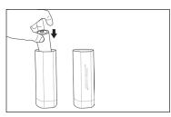
2. In the left compartment insert 2 C-cell batteries with the negative side down.
