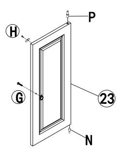
Note:Put the P part to the hole first and then put the N part
