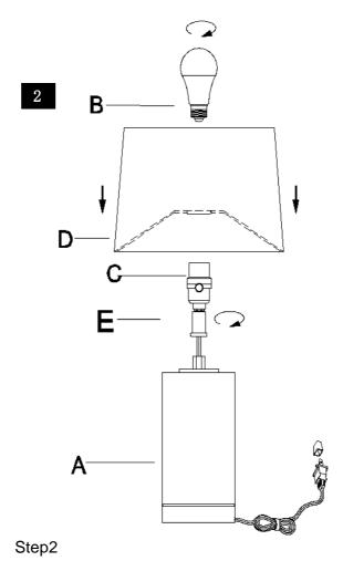
Put the shade(D) on the Scoket(C),then Screw the Bull (B)into the Scoket (C)
