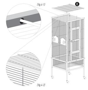
When all extended wires and corresponding holes are aligned, secure the **center top** [C] panel with a long hex screw in each corner.
