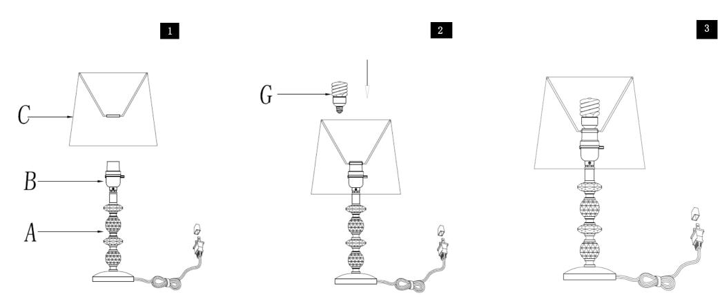
Step 1 Unpack all parts from cartons carefully Put the shade(C) on the Socket(B), then
