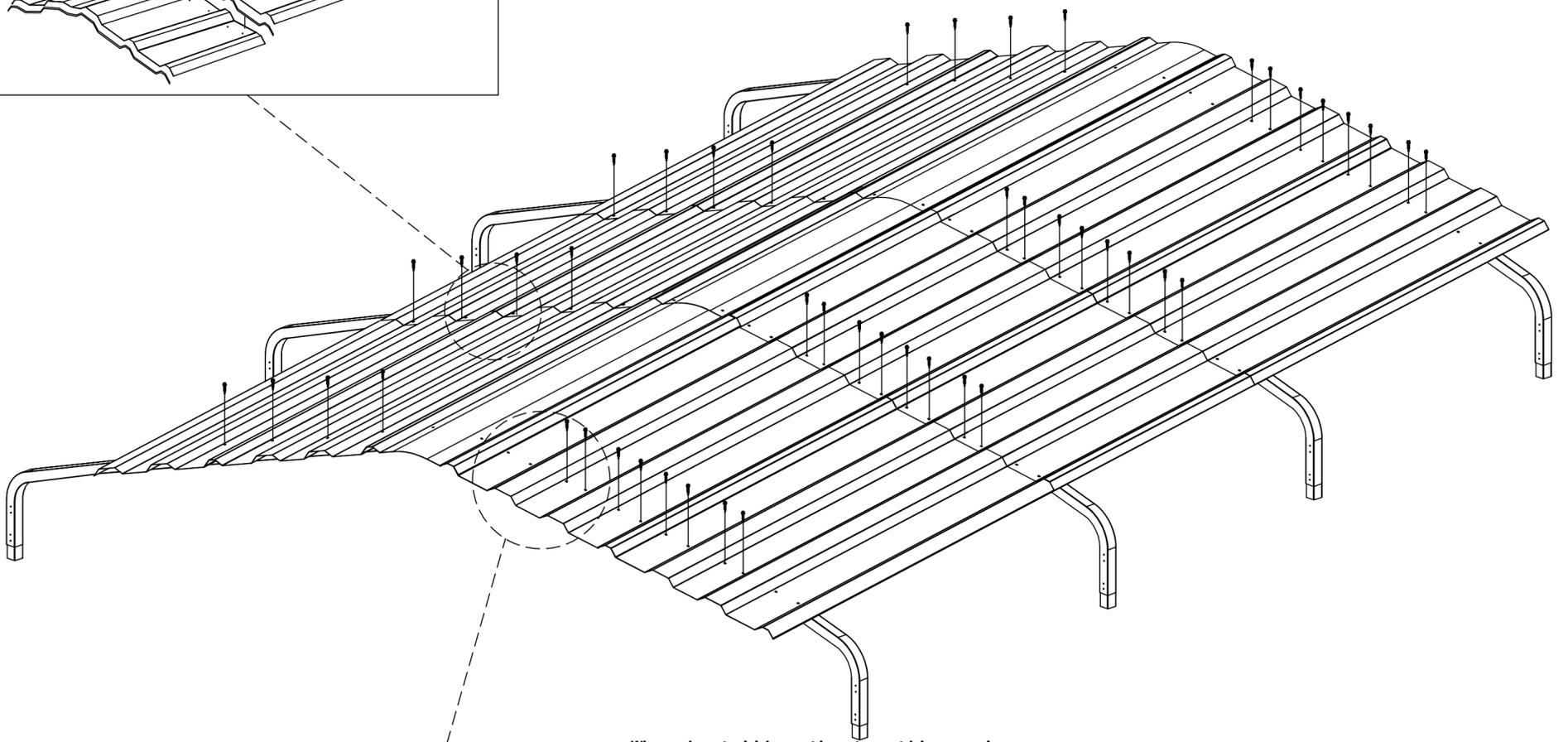
When installing the top tiles, please note that the upper tiles must be pressed against the lower tiles to avoid water ingress.
