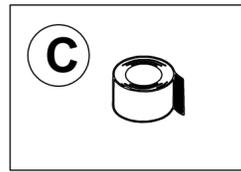
Stick the waterproof strip on the iron pipe, do not cover the screw holes.
