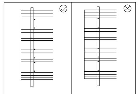
The position of the top tile installation should be 8 cm beyond the column.
