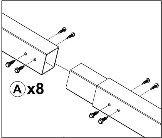
Connect the fittings with screws as shown in the figure
