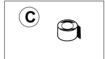
Stick the waterproof strip on the iron pipe, do not cover the screw holes.
