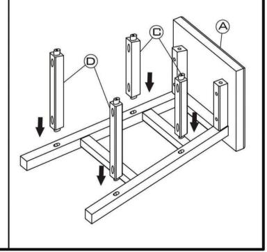
Attach the second leg assembly (B) to stool top (A), short stretchers (C) and long stretcher (D).
