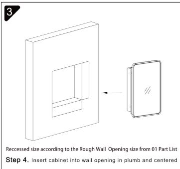
Step 4. Insert cabinet into wall opening in plumb and centered position. Use a carpenter's level and shim corners of cabinet if necessary.Step 5. Once cabinet is inserted into wall, measure down 4" from
