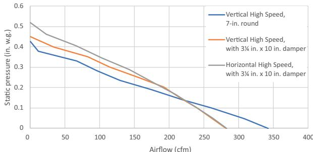
HVI-2100 CERTIFIED RATINGS comply with new testing technologies and procedures prescribed by the Home Ventilating Institute, for off-the-shelf products, as they are available to consumers. Product performance is rated at 0.1 in. static pressure, based on tests conducted in AMCA's state-of-the-art test laboratory. Sones are a measure of humanly-perceived loudness, based on laboratory measurements.
