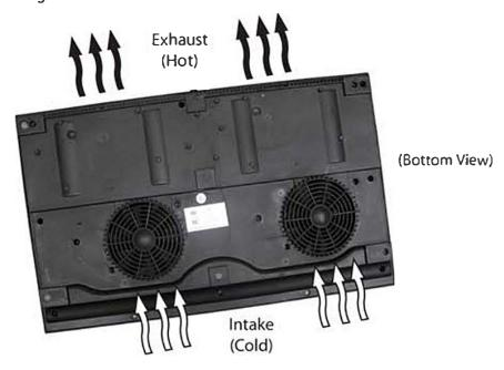
• For proper air circulation, allow at least 3" of clearance from the bottom of the induction cooker to any shelving or storage. The underside of the countertop should not be closed off from the cabinetry underneath for better air flow.
