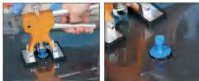
5. Place the dent lifter 6. Attach the puller tabs to the depression, wait about 2 minutes
