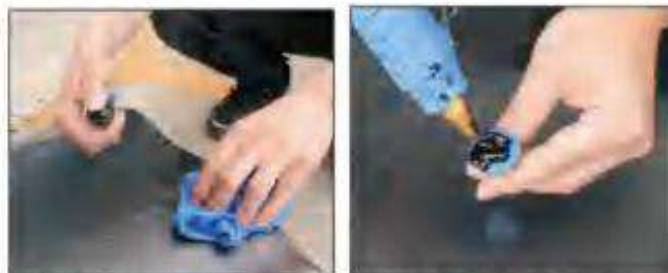
1. Clean the surface of the depression 2. Heat the glue stick with a glue gun and apply it to the puller tabs
