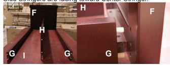
**Step 3:** Insert Threaded Cams (A) into holes in Side Stringers and Center Stringer. Turn so that the larger line is horizontal. Insert Large Bolts (C) into Table Leg (F) and thread into Cams (A). Do not overtighten.
