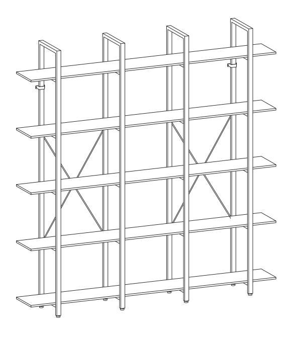
■ Please don't tighten the screws completely and go back later for a final tightening of all the screws after pieces are aligned with each other.
