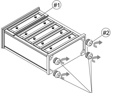
Insert the threaded end of the legs (#2) into the pre-drilled holes located on the bottom of the chest (#1). Tighten clockwise by hand.
