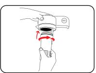
4. Attach the Filter Basket to the Control Lid by inserting it into the bottom of the Control Lid and turning clockwise until it is secure and no longer spins.
