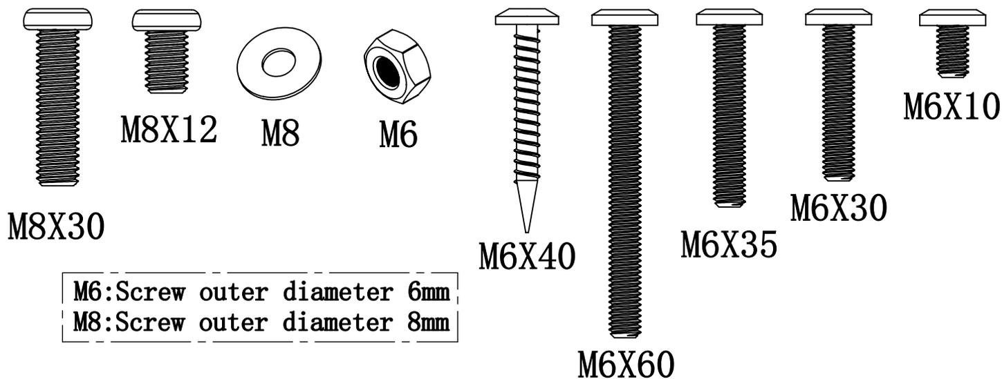
M6:Screw outer diameter 6mm
