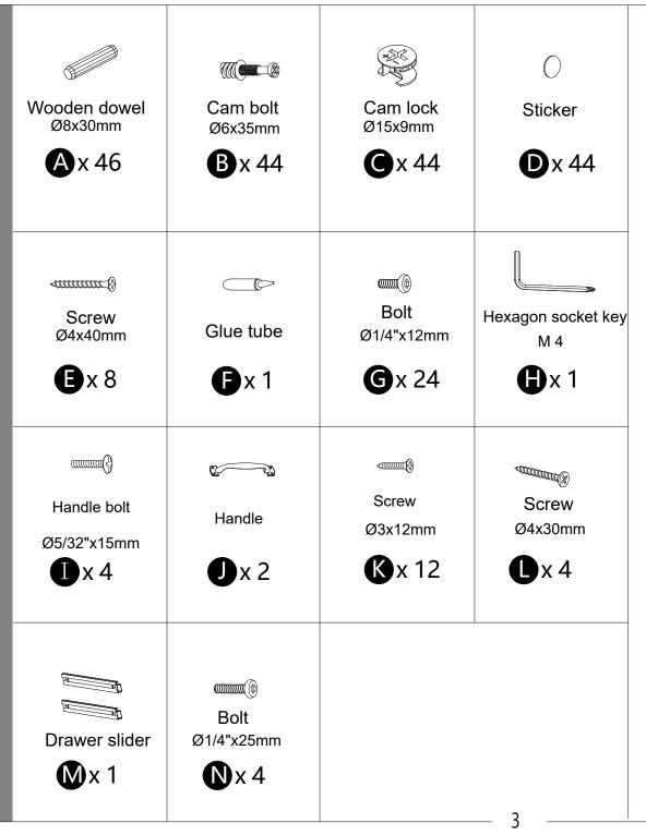
• The provided glue(F) is to secure wood dowels(A) in place. When first inserting dowels, locate the appropriate hole for the dowel, place a small amount of glue in the hole and insert the dowel. Wipe away excess glue immediately.
