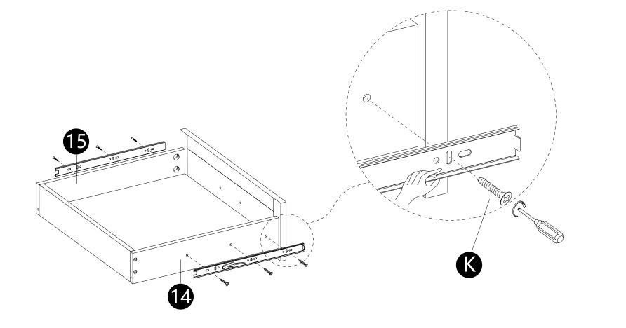
· Attach slider brackets to panels (14,15) with screws (K) correctly.
