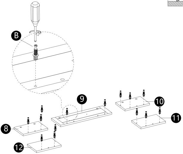
· Screw Cam bolts (B) into panels (8,9,10,11,12).
