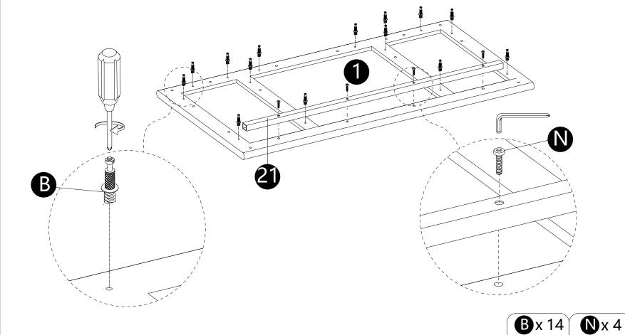
Screw Cam bolts (B) into panel (1).
