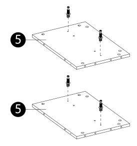
· Screw Cam bolts (B) into panels (4,5).
