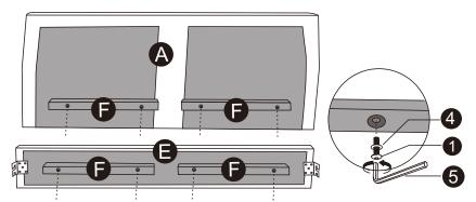
**STEP 3:** Attach the back and front rail bars (F) to the back frame(A) and front rail with bolts (1), washer(4) and allen key (5)
