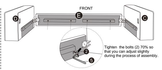
**STEP 4:** Attach front rail (E)to ammrests (C,D) with bolts (2) and allen key (5).
