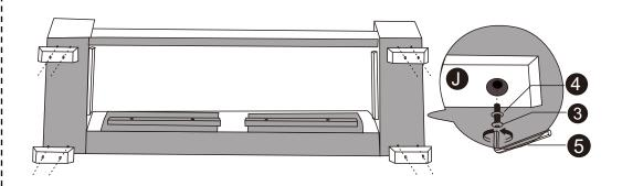
**STEP 6:** Screw legs(J) in to bottom of armrest with bolts(3), washer(4) and allen key(5).
