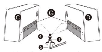
**STEP 2:** Attach the side rail bars (G) to the armrests(C,D) with bolts (1), washer(4) and allen key(5)
