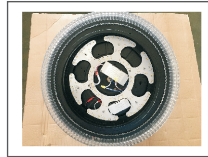
Step 4. The LED light source and the LED and Bluetooth integrated driver are mounted on the chassis by means of magnets.
