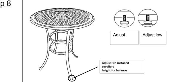
Adjust the Legs pre-installed Levellers until the Table is level with the ground.
