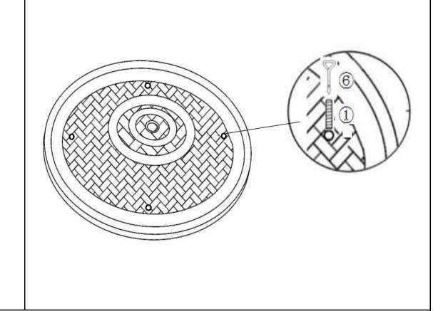
Lay the Table Top(A), facedown, onto a flat, soft, clean surface and lock the mounting positions with bolts(1) by using screwdriver(6).
