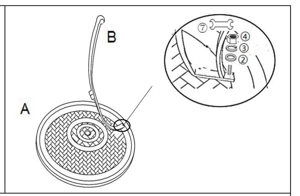
Attach the Table Leg with pre-attached Leveller(B) to the Table Top(A) with washers(②),spring washers(③),and nuts(④) using spanner(⑦). **DO NOT OVERTIGHTEN.**
