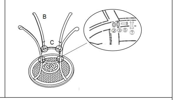
Loosely attach the Round Support (C) to Table Leg with pre-attached Leveller(B) with washers(2), spring washers(3) and hex nuts(5) using spanner(7).
