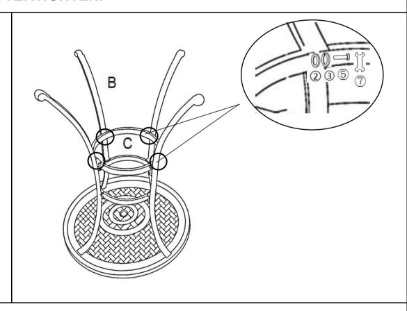
Loosely attach the Round Support (C) to Table Leg with pre-attached Leveller(B) with washers(2), spring washers(3) and hex nuts(5) using the spanner(7).
