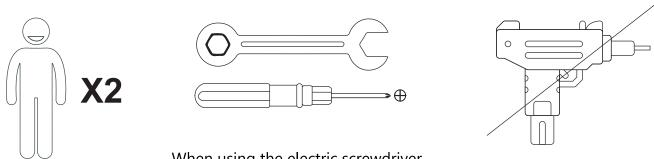
When using the electric screwdriver, Reduce the power and torque to avoid damaging the furniture
