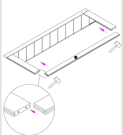
Gently slide slats X1 to X5 into the left side of L2 with all their grooves facing up. Make sure all the slats following the direction in instruction.
