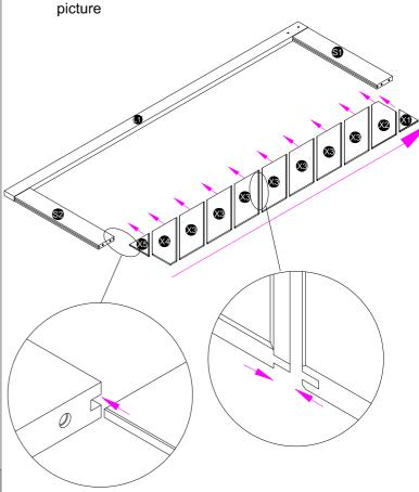
Insert middle stile (L2) into frames in the direction of instruction. Make sure every slat is in right position.
