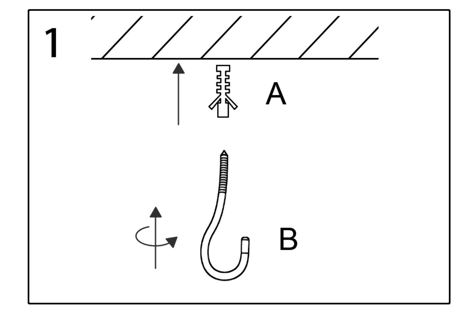
1.Drill a hole with impact bit machine at the ceiling, hit the expansion anchor into the hole with hammer, rotate to install the ceiling hook to the anchor.
