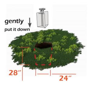
Make sure the inground base is horizontal. Backfill the hole with at least 700 lbs of concrete.
