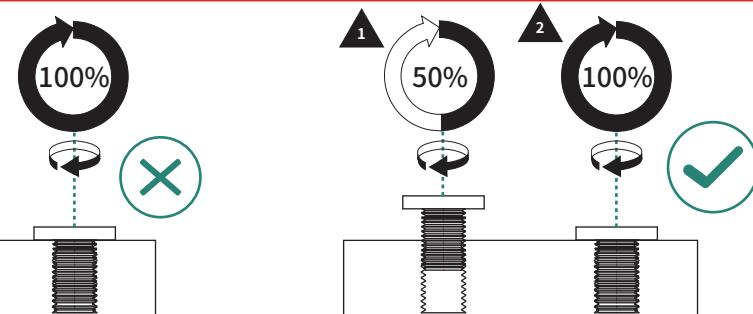
1. First, partially tighten all the screws to about 50% of the full torque, do not fully tighten them.
