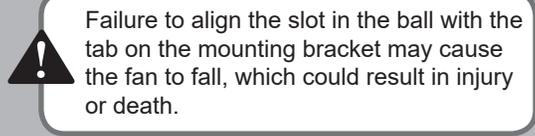
Failure to align the slot in the ball with the tab on the mounting bracket may cause the fan to fall, which could result in injury or death.
