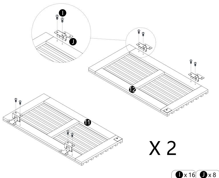
$\cdot$  Attach parts (J) to panels (11,12) with screws (I) correctly.
