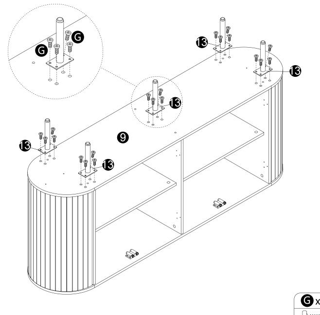
· Attach parts (13) to panel (9) with screws (G) correctly.
