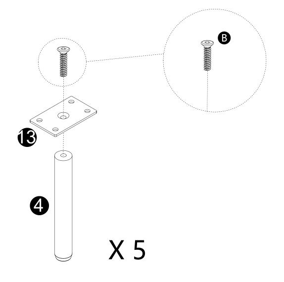
· Attach parts (13) to parts (4) with Bolts (B) correctly.
