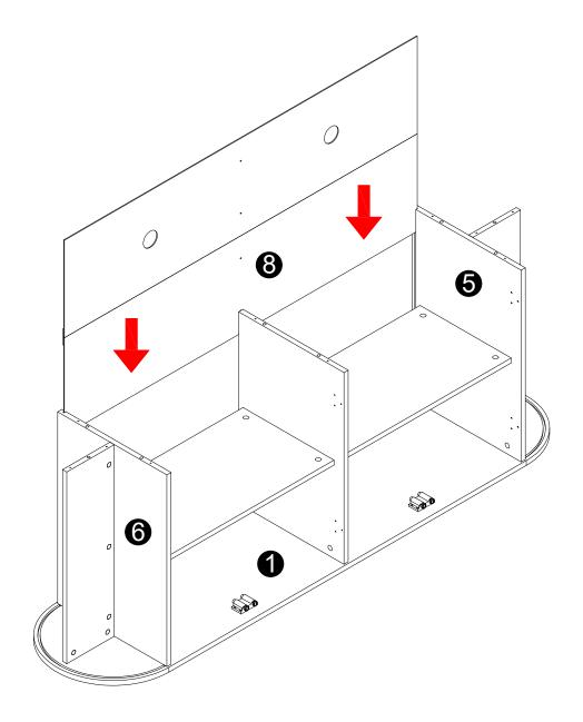
$\cdot$  Carefully slide panel (8) into place along the back of the assembly.
