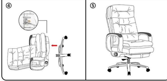
4. Insert the top of the gas lift cylinder into the mounting hole.
