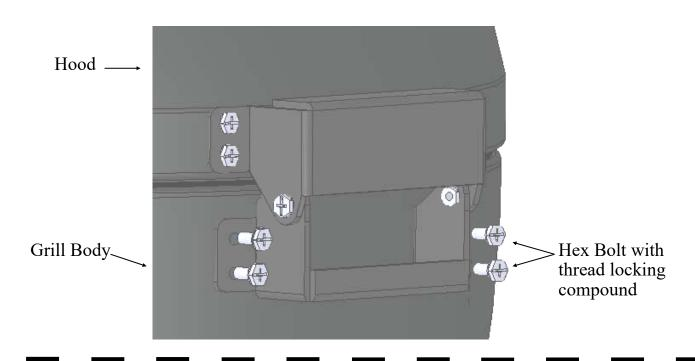
Attach FRONT HANDLE to HOOD with four (4) 1/2 inch hex bolts. First attach one HANDLE BRACKET to the Lid and then hold the HANDLE in place while attaching the other HANDLE BRACKET to the Lid. HANDLE BRACKETS are left and right handed.
