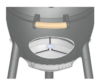
Position O-Ring on bottom of damper by rolling it up to the bead. With O-Ring in position, install DAMPER with two (2) 1/2 inch bolts from inside the HOOD. Damper coating will scratch with use. This does not affect the function or performance of the damper. Next, install THERMOMETER GASKET, THERMOMETER, and BEZEL with wing nut, as shown below.
