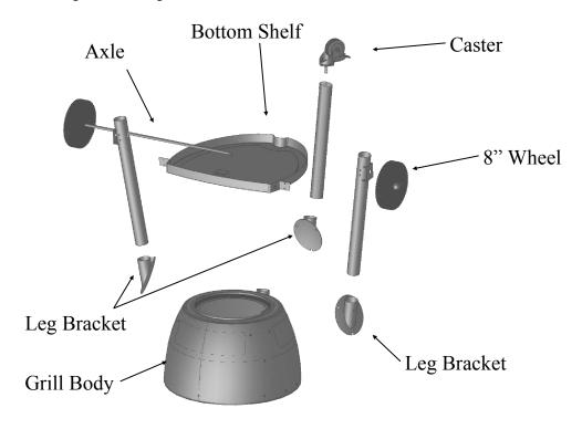
**Step 2**Attach BOTTOM SHELF to LEGS with five 1/2 inch hex bolts and lock washers.
