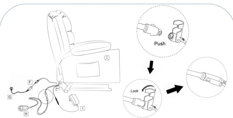
The pins must be connected correctly.
