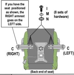
Using screws (J), O 'rings (M) and washers (N), assemble the backrest (A) to the metal brackets on the seat (B) as shown.
